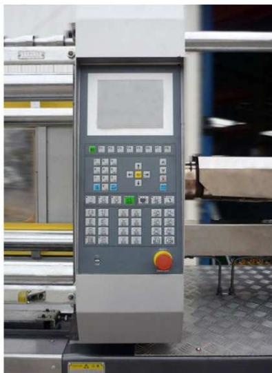
CPU controller and display are independent and reliable. A larger Color LCD screen enhances clear display and supports multi-language compatibility. The control system also supports remote monitor. In the event of a control problem, the machine can be connected to internet through a special interface. Dakumar service can realize remote fault diagnosis and maintenance.
